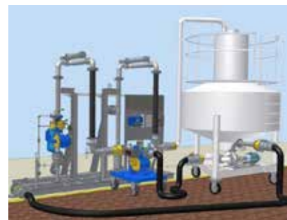
Fig.3: Master Meter with proving tank
